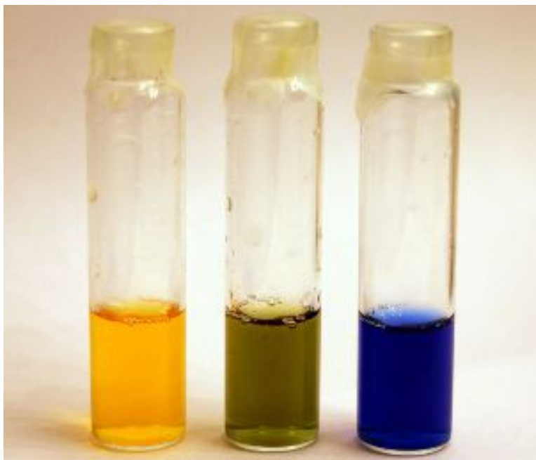
Figure 5.5: Bromothymol blue (BTB) changes from blue to green to yellow as carbon dioxide is added. Thus, it is a good indicator for this product of burning or cellular respiration.
