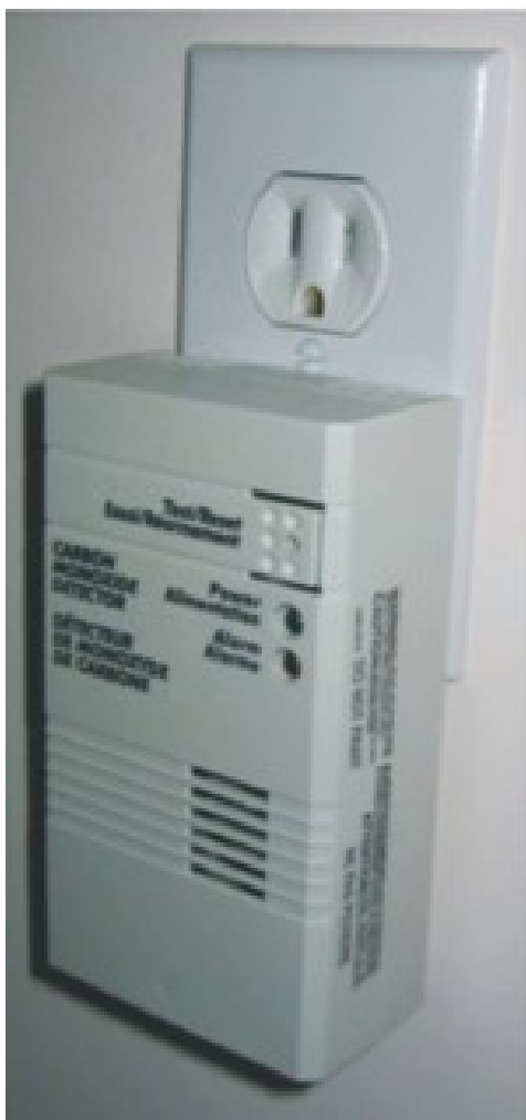
Figure 24.15: Home carbon monoxide detector
