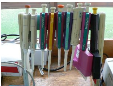
Figure 1.29: Pipettes are small, but important tools in many biology labs. Micropipettes, such as these here, are calibrated to measure very small amounts of liquids. For example, 100 microliters (100 \mu\text{L} ) which is about half the volume of your little finger tip; or even 1 \mu\text{L} , which is smaller than a drop of water.
