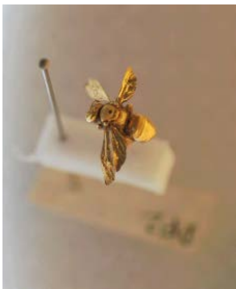
Figure 1.33: This insect has been coated in gold, as part of the preparation for viewing with an SEM.
