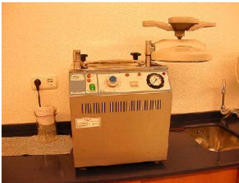
Figure 1.35: A worktop autoclave. Autoclaves commonly use steam heated to 121^{\circ}\text{C} ( 250^{\circ}\text{F} ), at 103\text{ kPa} ( 15\text{ psi} ) above atmospheric pressure. Solid surfaces are effectively sterilized when heated to this temperature. Liquids can also be sterilized by this process, though additional time is required to reach sterilizing temperature.
