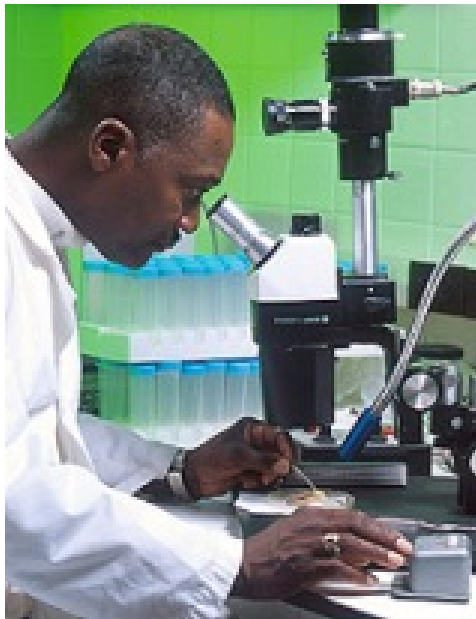
Figure 1.31: This scientist is using a stereo microscope, which is a light microscope with two ocular lenses (the microscope lens that is closest to the eye). The microscope is fitted with a digital imaging device that can take digital photos of what the researcher sees.
